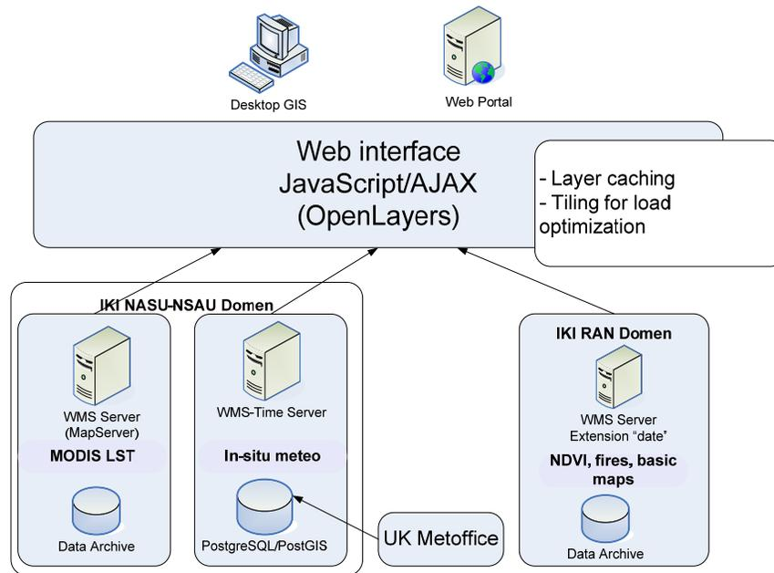
Figure 11. Architecture of satellite monitoring system integration
