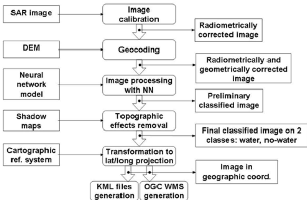
Figure 3. Flood mapping from SAR satellite imagery: workflow
