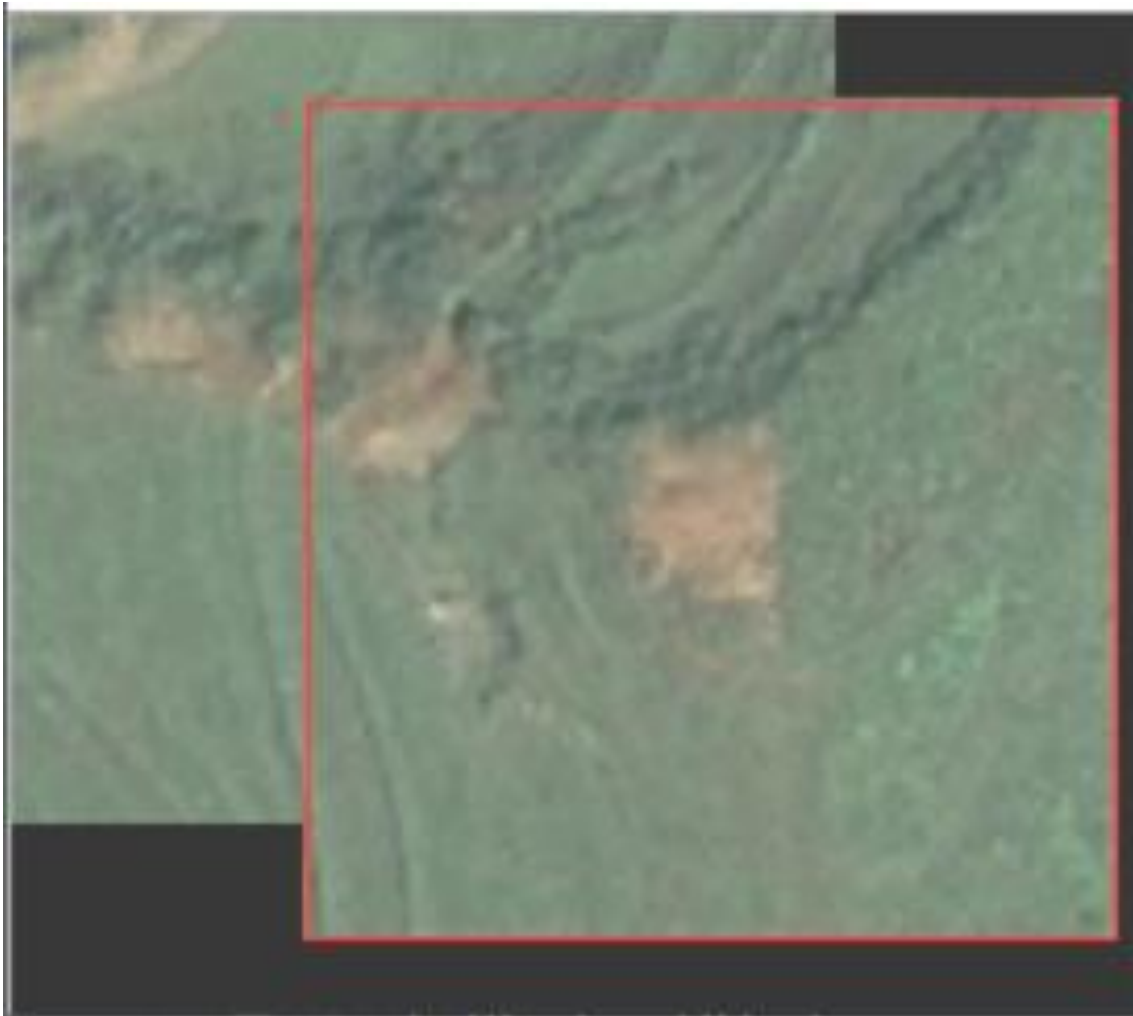
Fig. 4 Photo from the UAV superimposed on a satellite the area photo as an example of the program operation for combining two photos using OpenCV (an open source computer vision library available for free use for scientific, academic and commercial purposes).
