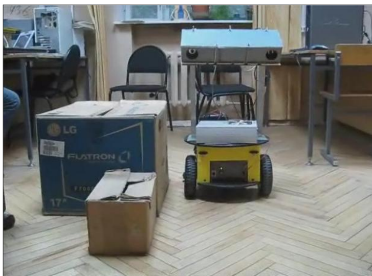
Fig. 2. Mobile robot equipped with the 3D computer vision system in experiment.
