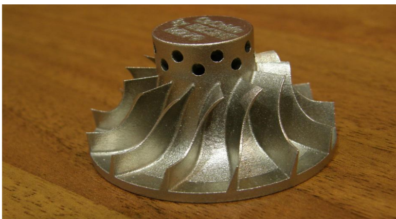
Figure 3. Rotor made by SLS method
