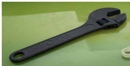
Figure 6. Element produced by PolyJet method
