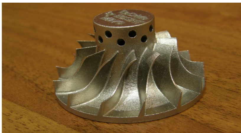
Figure 3. Rotor made by SLS method
