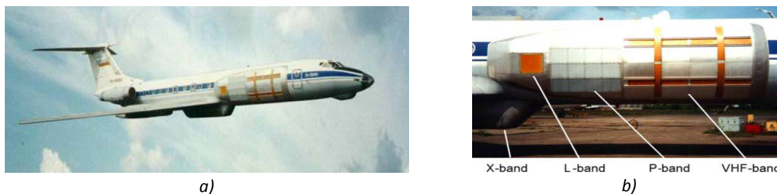
Figure 132. "Flying MCW Laboratory (a) and allocation of special antennas on the airplane (b)
