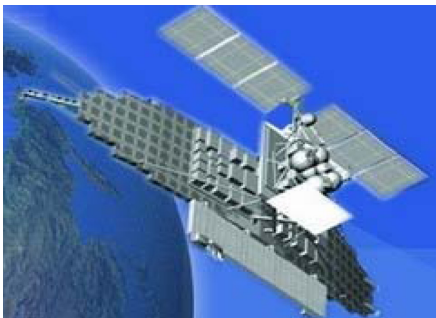
Figure 134. Example of dual-frequency spaceborne radar with synthetic aperture
