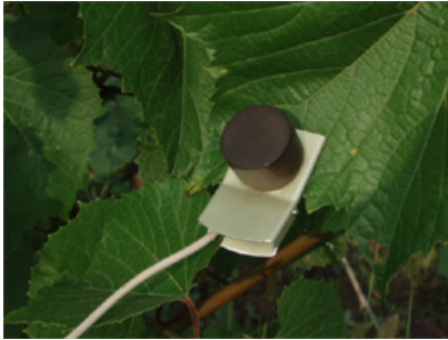
Figure 71. The sensor of the "Floratest" on the vine leaf Figure 72. The image of CFI on the device's display
