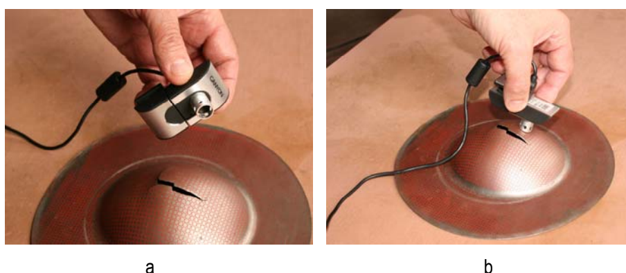
Fig. 5. a – A view of the CCD camera, equipped by mechanical piece; b – The optical sensor in a process of manual scanning.
