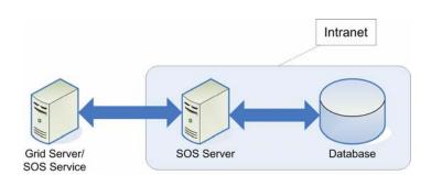
Fig. 3. Grid-based SOS service implementation
