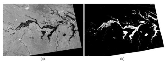
Fig. 4 Raw ENVISAT image (a) and resulting flood extent shown with white color (b) for Huaihe river, China (© ESA 2007)
