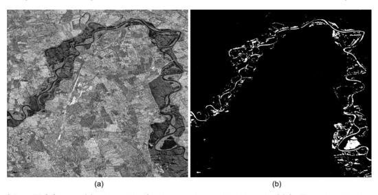
Fig. 3 Raw ERS-2 image (a) and resulting flood extent shown with white color (b) for Tisza river, Ukraine and Hungary (© ESA 2001)
